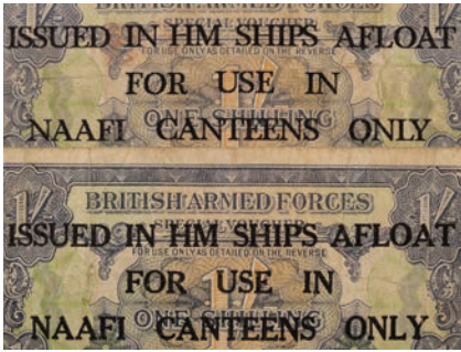
Above: A fraudulent inkjet “overprint” (top) applied to raise the value of the underlying military note. The L extending under the left arm of the Y in ONLY could be done only digitally, not with conventional printing type.
