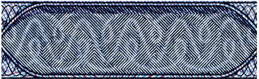
Above: The latent image of "১০০" (100 in Bengali numerals) from a banknote issued by the Bangladesh Bank. This illustrates how the latent image is created by lines of intaglio ink being printed in two directions. The lines of the background are printed from top left to bottom right, while the lines creating the numerals are printed from the top right to bottom left.
