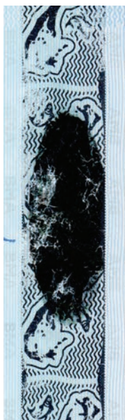
Left: To counter the advantage of a clear window on polymer notes, manufacturers of paper notes created banknote paper with holes in them, then covered the holes with plastic strips, creating a clear window – shown here by the black background. These became known as "hybrid" notes, as seen on this detail in a banknote from Bermuda.
