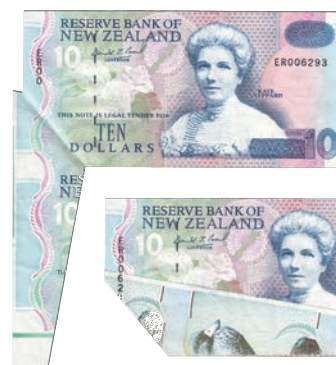
This error was caused by a fold in the paper, after the banknote sheets were printed but before the serial numbers were printed and the sheets guillotined. This creates a "flap."
