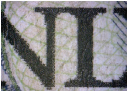
Above: Inkjet printing. Note the stair steps on the diagonals and curves. Digital processes do not always handle angles well. Note also the left arm of the Y extending into the L's space at right.
